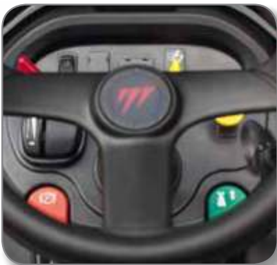
Dash board: cruise control and RMO (Reverse Mow Option).
